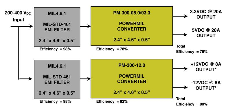
\*Note 1: All PowerMil outputs are isoalted from the input, chassis, and its adjoining outputs. The outputs are floating and can be used as plus or minus outputs.
